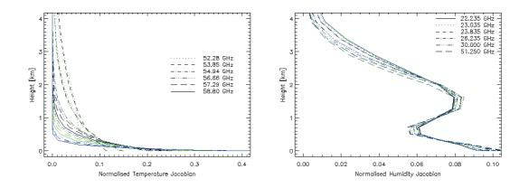
Figure 5-5 Normalised Jacobians showing sensitivity of Radiometrics TP/WVP-3000 channels viewing at zenith angles,  $\theta$ =0° (black), 60° (green) and 75.5° (blue) for temperature (left) and humidity (right).
