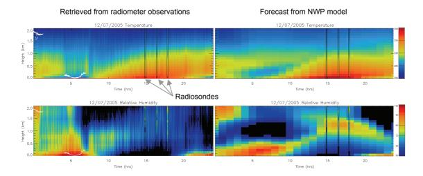
Figure 6-12 Time-height plots of temperature [K](top) and relative humidity [%](bottom) retrieved from radiometer observations (left) and hourly T+0 to T+24 hr forecasts (right) from mesoscale version of the Met Office Unified Model for Linkenholt on 12/7/05.
