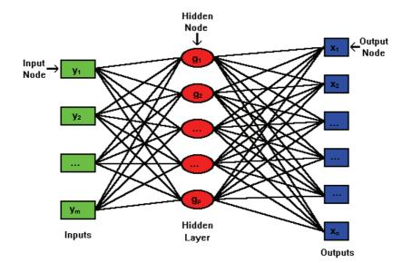
Figure 5-1 Schematic diagram showing a Neural Network with 1 hidden layer fully connected between a set of input nodes, y, and output nodes, x.
