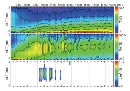
Figure 6-1 Time-height plots of profiles retrieved from radiometer observations at Cardington over 12 hours on 8/4/03. Upper panel shows temperature (°C), middle panel shows relative humidity (%RH), lower panel shows liquid water content (g/m<sup>3</sup>). Vertical lines indicate times of radiosondes plotted in Figure 6-2.
