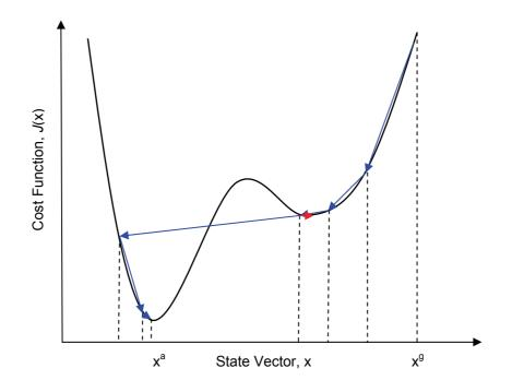
Figure 4-14 Schematic of minimisation of nonlinear cost function by Levenberg-Marquardt method, showing state vector, x, at each iteration (blue arrows) from first guess, x<sup>9</sup>, to analysis, x<sup>a</sup>. Red arrows are iterations that fail to reduce cost function, *J*.
