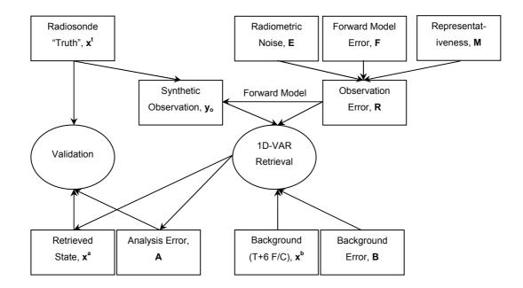
Figure 4-18 Schematic 1D-VAR with synthetic observations and background from T+6 hr forecast from NWP model
