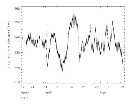
Figure 6-10 Time series of 1000-500 hPa thickness calculated from profiles retrieved by neural network from radiometer observations at Cardington in Spring 2003.
