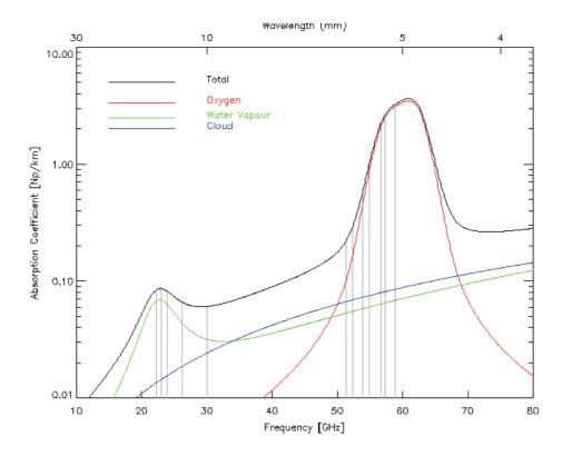
Figure 1-1 Atmospheric absorption spectrum for typical surface conditions: *T*=288.15 K, *p*=1013.25 hPa, *RH*=100%, *L*=0.2 g/m<sup>3</sup> following Rosenkranz [1998]. Lines show total absorption coefficient and contribution from oxygen, water vapour and cloud, coloured according to the legend. Grey vertical bars indicate the centre frequencies of the Radiometrics TP/WVP-3000 microwave radiometer.
