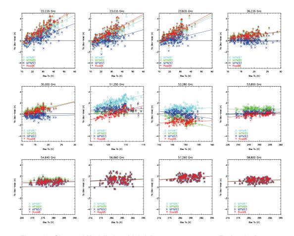
Figure 3-4 Observed-Modelled zenith brightness temperatures. Each point is one radiosonde, modelled using MPM87(△), MPM89(◊), MPM93(x), Ros98(+).
