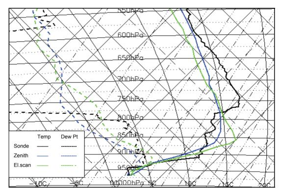
Figure 6-8 Tephigram showing profiles of temperature (solid line) and dew point (dashed lines) in lowest 5 km at 1100 UTC on 5/12/03 at Payerne, Switzerland. Black lines show profile from radiosonde.
