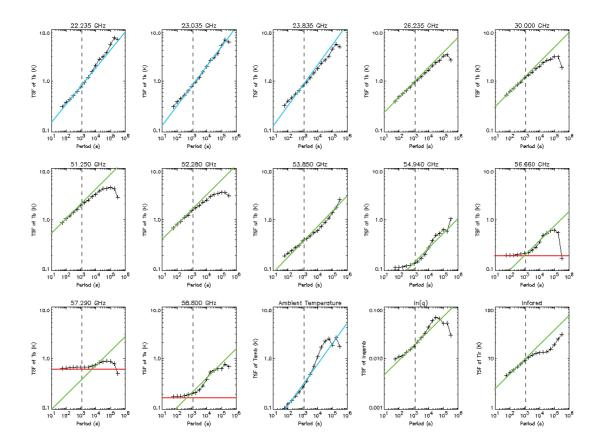
Figure 4-6 Time Structure Functions of Radiometrics TP/WVP-3000 observations measured at Camborne 23-29 July 2004 in all dry conditions. Coloured lines show reference slopes: Red=0, Blue=1/3, Green=1/4.
