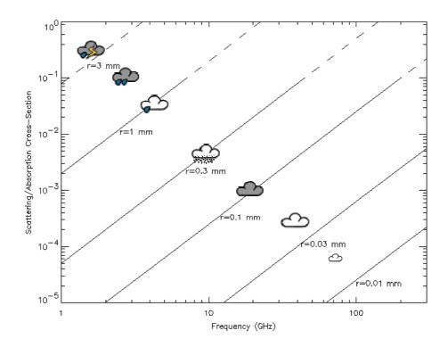
Figure 1-2 Ratio of scattering to absorption cross-sections for water spheres radius, *r*, at microwave frequencies. Typical drop sizes are indicated ranging from small and large cumulus clouds, drizzle, light rain, heavy and torrential rain. Solid lines indicate where Rayleigh scattering criterion is valid  $2\pi r <<\lambda$ . Dashed lines indicate the transition to the Mie scattering regime. Adapted from Janssen [1993].
