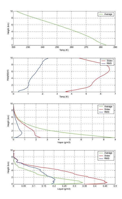
Figure 5-2 Average and standard deviation (Stdev) of 10 year radiosondes from Camborne used to train the neural network and r.m.s. error (RMS) of its retrievals. [Courtesy of Radiometrics]
