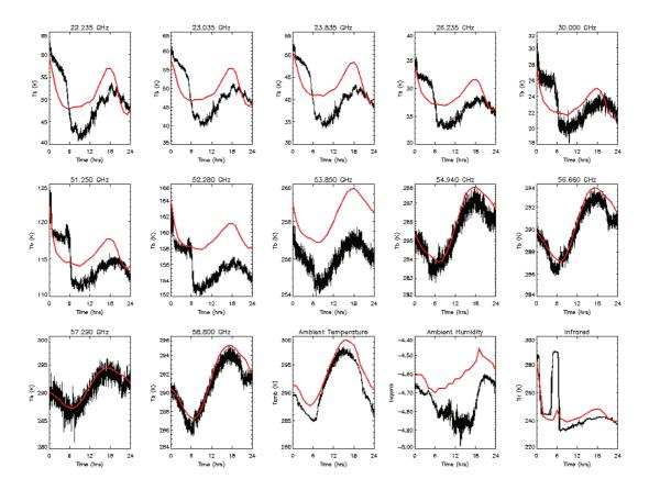
Figure 6-13 Time series of observations from Radiometrics TP/WVP-3000 (black) and forward modelled mesoscale model output (red) from 00-24 UTC on 12/7/05 at Linkenholt.
