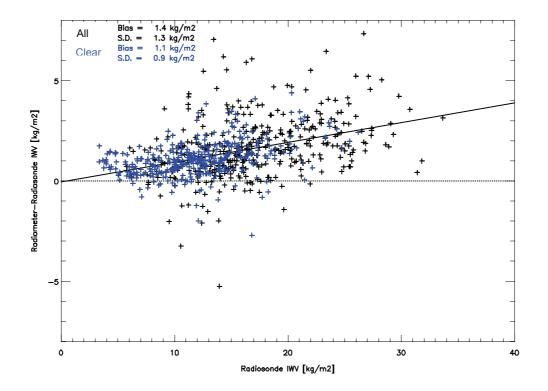
Figure 5-7 Difference between IWV retrieved using neural network and calculated from radiosonde profiles at Camborne 20/2/02-18/3/03. Solid line shows best fit by linear regression. Black crosses are all cases, Blue crosses are the subset of clear cases.
