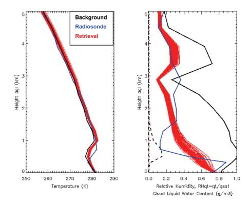
Figure 4-22 Example retrievals (red) with 105 synthetic observations, with profiles between NWP model background (black) and radiosonde (blue). Left panel shows temperature profiles. Right panel shows profiles of relative humidity ( $RH_{qt}=q_t/q_{sat}$ ) and cloud liquid water content [g/m<sup>3</sup>] (dotted lines).
