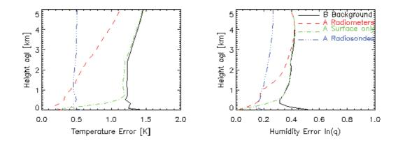
Figure 4-10 Error Analysis for 1D-VAR retrievals. Background error covariance matrix from mesoscale model, √diag(B<sub>ATOVS</sub>) (black) and analysis error covariances matrices, √diag(A), with surface sensors only (green), radiometers and surface sensors (red), and radiosonde only (blue). Diagonal components plotted for lowest 5 km of temperature [K] and humidity (*Inq*).
