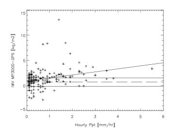
Figure 5-9 Bias in IWV retrieved with Radiometrics TP/WVP-3000 neural network relative to GPS compared to precipitation rate for all wet hours during TUC. Horizontal lines show mean and standard deviation of the difference in IWV during dry conditions. Sloping line indicates linear regression of observations.
