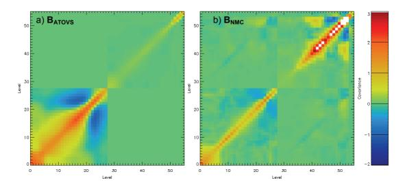
Figure 4-3 B matrices used in assimilation of ATOVS satellite data in the northern hemisphere by Met Office 1D-VAR, interpolated to lowest 28 UMG3 levels (left) and calculated by NMC method using T+6 – T+12 mesoscale model forecast profiles for Larkhill over 1 year (right). The state vector comprises temperature [K] at 28 levels, followed by total water (lnq<sub>t</sub>) [dimensionless] at the same 28 levels.
