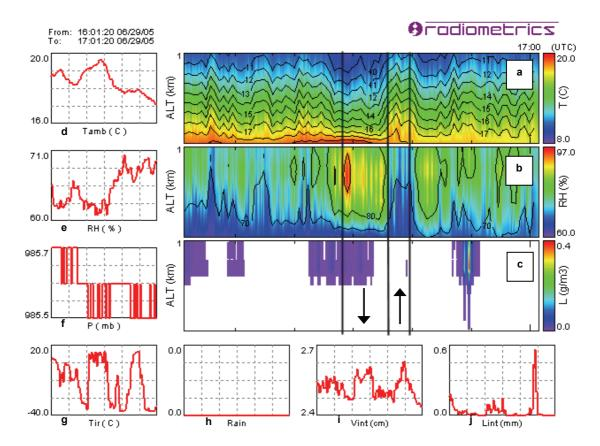
Figure 6-5 Retrievals from microwave radiometer observations on 29/6/05 16-17 UTC showing (a) temperature, (b) relative humidity and (c) liquid water time-height cross sections for 0-2 km height. Time series of scalars are also shown in red for (d) surface temperature, (e) surface relative humidity, (f) pressure, (g) infrared brightness temperature, (h) rain sensor, (i) integrated water vapour and (j) integrated liquid water. Arrows indicate updraught and downdraught.
