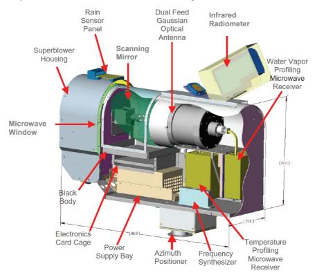
Figure 3-1 Cut-away Diagram of Microwave Radiometer TP/WVP-3000 System [Courtesy of Radiometrics]
