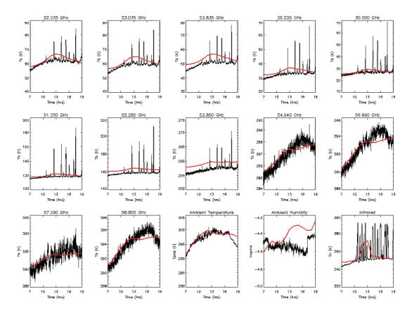
Figure 6-15 Time series of observations from Radiometrics TP/WVP-3000 (black) and forward modelled mesoscale model output (red) from 07-19 UTC on 13/7/05 at Linkenholt.
