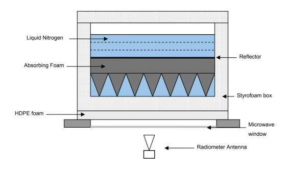
Figure 3-3 Cryogenic Target used to Calibrate  $T_{ND}$  for 51-59 GHz channels.
