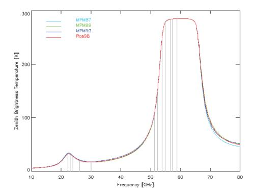
Figure 2-2 - Spectra of zenith brightness temperatures for clear standard atmosphere modelled with MPM87, MPM89, MPM93 and Ros98 absorption models. Vertical grey lines indicate centre frequencies of Radiometrics TP/WVP-3000 channels.
