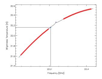
Figure 2-3 –  $T_b$  spectrum near 22.235 GHz channel of Radiometrics TP/WVP-3000. Calculated using Ros98 for 1976 US Standard Atmosphere in zenith view. Red crosses indicate the passband of the 22.235 GHz channel. Blue cross shows  $T_b$ evaluated at the channel's centre frequency. Blue diamond shows the band-averaged
