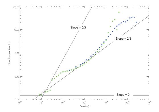
Figure 5-8 Time Structure Functions of IWV (kg/m<sup>2</sup>) retrieved from Radiometrics TP/WVP-3000 (blue) and WVR1100 (green) during Cardington trial of Spring 2003. Lines show theoretic slopes of 2/3 and 5/3, and 0 (instrument noise).
