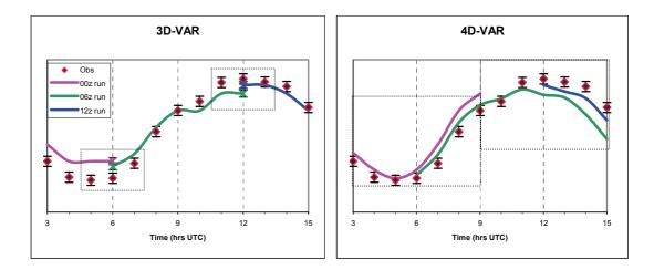
Figure 1-3 Schematic diagrams showing process of assimilating hourly observations (points with error bars) in boxed windows using previous model run as background.
