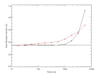
Figure 3-6 Time structure functions of 58.8 GHz  $T_b$  over 1106-1306 UTC during CSIP: 21/7 – 31/7/05 with calibration against ambient black body every 30 s (black), 26/6 – 7/7/05 without calibration, but sampled every 12s (red) [multiplied by  $\sqrt{2}$ ]. Horizontal line indicates white noise level on calibrated brightness temperatures.
