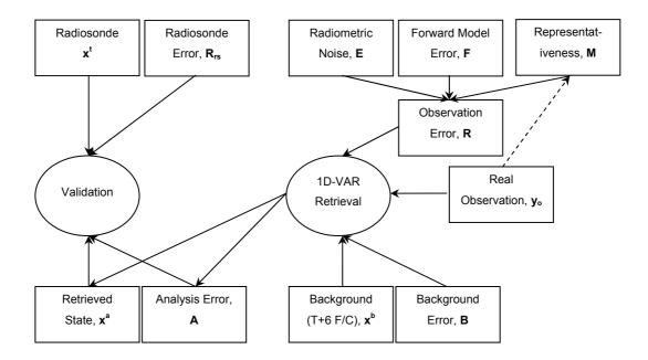
Figure 4-20 Schematic 1D-VAR with real observations and NWP background. (Dashed arrow indicates time series of observations used to calculate M dynamically.)
