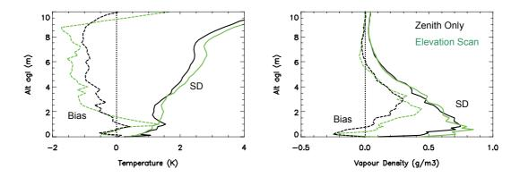
Figure 5-6 Statistics of neural net retrievals at Payerne 6/11/03-13/2/04, 165 cases. Solid lines show standard deviation of retrieved-radiosonde profiles. Dashed lines show mean bias of retrieved-radiosonde profiles. Retrievals from zenith views only (black) and elevation scans (green).
