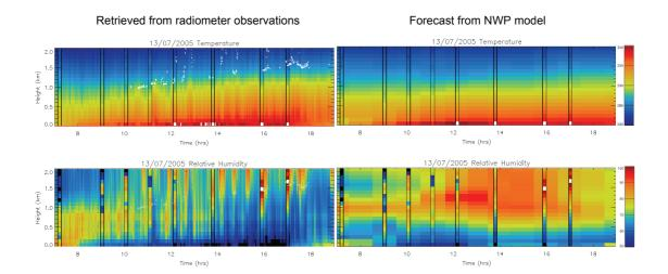
Figure 6-14 Time-height plots of temperature [K](top) and relative humidity [%](bottom) retrieved from radiometer observations (left) and hourly T+6 to T+18 hr forecasts (right) from mesoscale version of the Met Office Unified Model for Linkenholt on 13/7/05.
