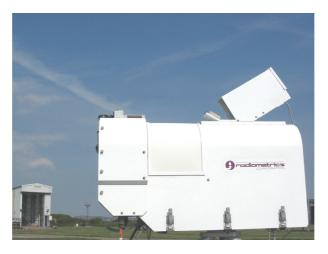
Figure 1-4 Radiometrics TP/WVP-3000 Microwave Radiometer System at Camborne.
