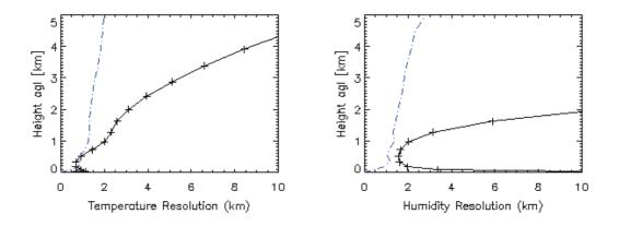
Figure 4-12 Vertical Resolution, ∆z, of temperature and humidity (In*q*) from microwave radiometer and surface sensors (black solid line) and radiosondes (blue, dashed line) in clear standard atmosphere using B<sub>ATOVS</sub>
