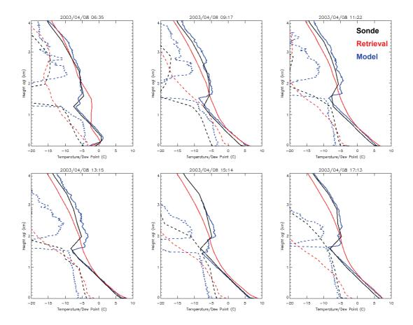
Figure 6-2 Profiles of temperature (solid lines) and dew point (dotted lines) measured by 6 radiosondes (blue), forecast from mesoscale NWP model (black) and retrieved from radiometer observations (red) at Cardington on 8/4/03.
