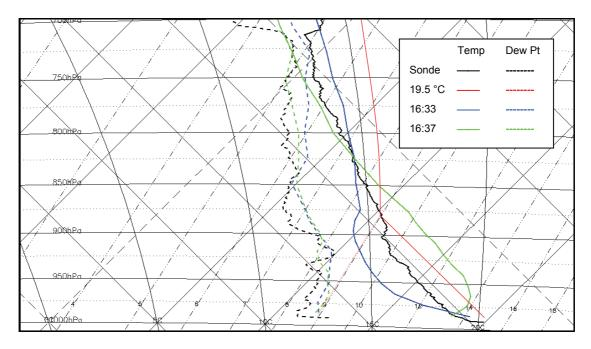
Figure 6-6 Tephigram showing profiles of temperature (solid line) and dew point (dotted lines) in lowest 3 km on 29/6/05. Black lines show profile from radiosonde launched from Larkhill at 1600 UTC.
