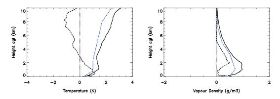
Figure 5-4 Statistics of neural net retrievals at Camborne 20/2/2002-18/3/2003. Retrieved profiles averaged within 30 min of radiosonde launch time. Black solid lines show Standard Deviation of retrieved-radiosonde profiles, Black dashed lines show mean bias of retrieved-radiosonde profiles, Blue dot-dash lines show r.m.s. residuals of neural network training. 1038 cases.
