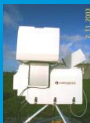
Figure 3. Liquid nitrogen calibration target [Courtesy of Radiometrics]
