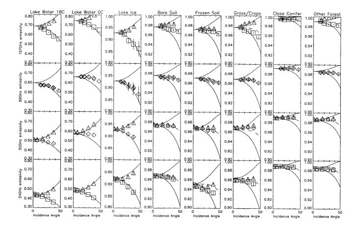
Fig. 1. Angular Variation of Emissivity. △: Vertical, □: Horizontal, ◊: Mixed Polarisation
