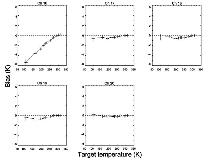
**Figure 2** Residual error in MARSS observations of earth target temperature, as a function of earth target temperature. Note channel 16 non-linearity leads to errors near  $5\text{K}$  for scene temperatures of  $100\text{K}$ .
