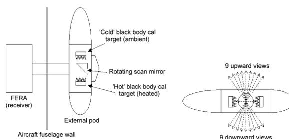
**Figure 1** MARSS configuration. Inside the aircraft, the FERA views the environment via a rotating scan mirror mounted in an external pod. The scanning mirror also provides views of black-body calibration targets, one at ambient temperature and one heated.
