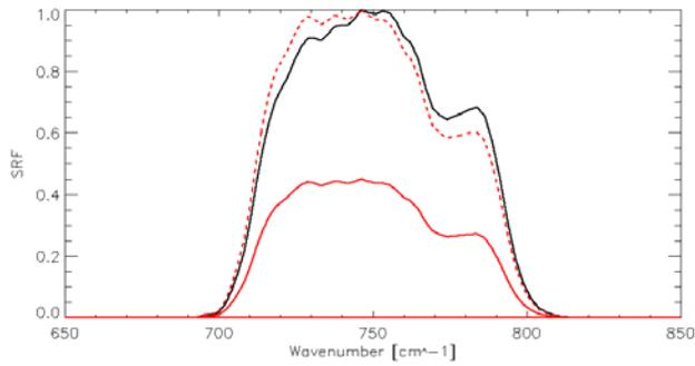
**Fig. 2. Spectral Response Functions of Meteosat-9 13.4  $\mu\text{m}$  channel:**
