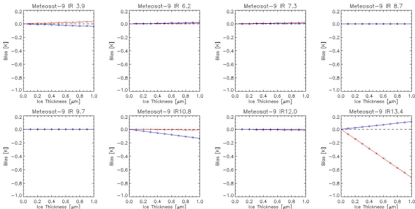
**Fig. 4. Bias in brightness temperatures modeled by modifying Meteosat-9's SRF by the transmittance of different thicknesses of ice. Solid lines show the predicted differences in brightness temperature compared with the uncontaminated instrument, accounting for calibration gain changes, based on calculation in US Standard Atmosphere with clear skies (red line with crosses) and thick cloud with tops at 194 hPa (blue line with diamonds).**
