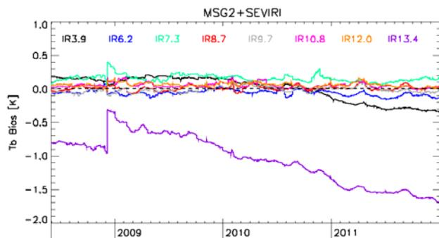
**Fig. 1. Example time series plot showing relative bias of IR channels of Meteosat-9/SEVIRI (MSG2) wrt Metop-A/IASI, expressed as brightness temperature difference for standard radiance scenes (corresponding to a 1976 US Standard Atmosphere with clear sky). A spacecraft decontamination in Dec 2008 reduced the bias of the 13.4  $\mu\text{m}$  channel, which subsequently continued to deteriorate.**
